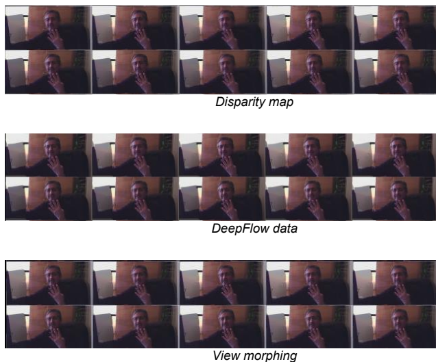
Figure 1: Example of intermediate views (e.g., positions from number 11 to number 20 in the Quilt) by morphing a stereoscopic image from L-to-R using our Morpholo library: (i) Upper set of images are generated via Disparity map, (ii) Middle images via DeepFlow and (iii) Lower images through View morphing.
