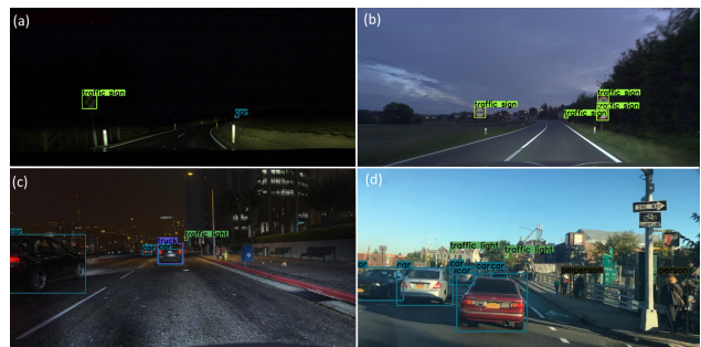
Figure 6. Object detection result of the final network on different images: (a) CVL, (b) GTSRD, (c) VIPER, and (d) BDD test datasets (not used for training).
