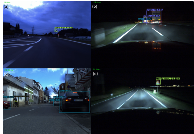
Figure 5. Examples of object detection results of the final network under different lighting conditions, with computed confidence values. The images shown were taken from the CVL test dataset.
