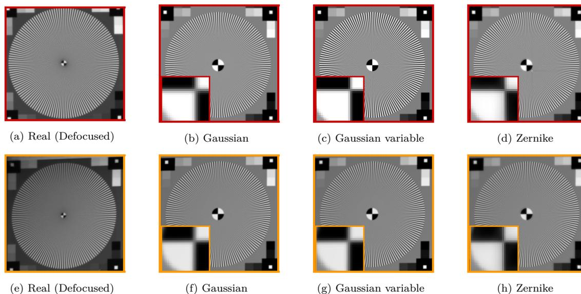
Figure 3: Harmonic Siemens Star from the center (upper row) and the upper left corner (lower row).
