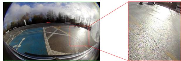
Figure 1: Illustration of sun glare causing perception issues. The zoomed in region shows wiping off lines.
