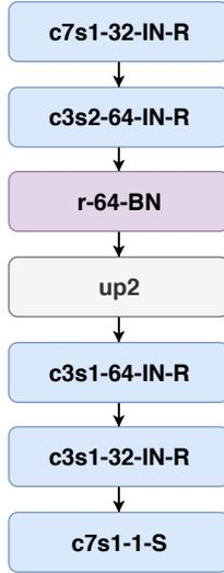
Figure 10: Proposed sun glare CNN architecture. Description of individual components is in the text.
