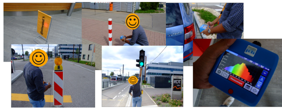
Figure 12: A measurement campaign with a JETI spectroradiometer 1511 [2] to obtain a set of typical spectra for automotive use cases.
