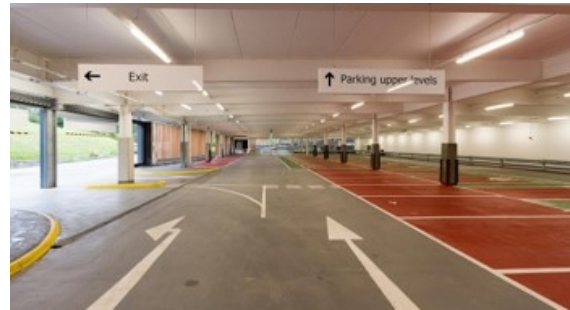
Figure 6: A typical scene when exiting a parking garage [11]. Many signs and lane markings need to be considered inside and outside the garage to have a full scene understanding. While inside the garage the luminance is low, outside the garage the luminance can be magnitudes higher. Consequently the lane contrast needs to be detected over a large dynamic range.
