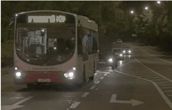
Figure 7. Example of HDR PWM flicker in lowlight scene. The bus sign is driven by a PWM signal. In this frame, the bus sign is captured only by the long exposure and missed by the short exposure. The combined output is a mid-grey artifact with no detail.
