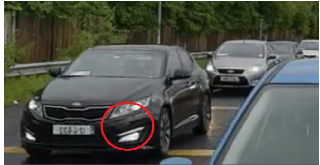
Figure 5. Example where LED flicker creates the impression that a vehicle's turn signal has been activated.
