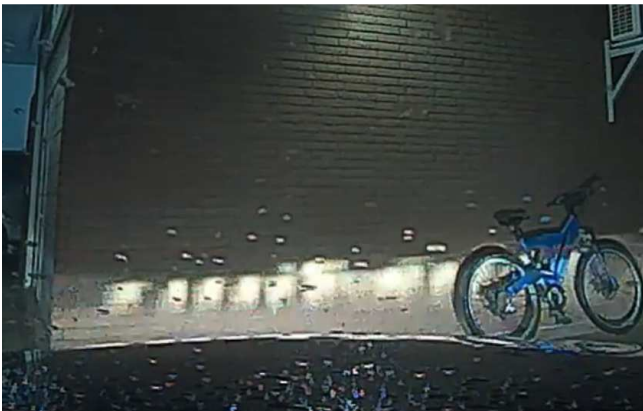
Figure 4. Example of LED artifact in rear view and/or surround view applications. In this example, the headlamps of the vehicle are reflected on the wall in front of the vehicle. The reflect light appears to flicker in a visually disturbing manner
