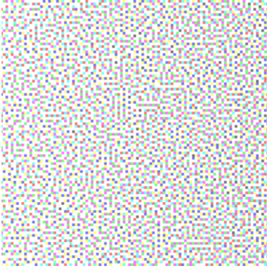
Figure 12. Halftoned image of Figure 9 using DBS screen blending-in and dot-off-dot 2-drop error diffusion algorithm.
