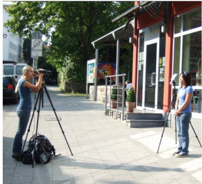
Figure 14: Capturing spectral data of natural objects with a tele-spectroradiometer. Here Skin tones and a white tile on the left side of the person to measure the characteristics of the illuminant.
