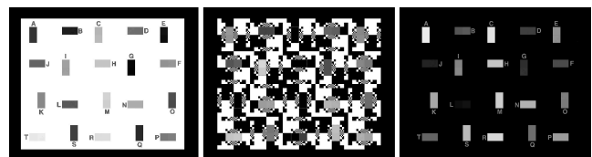
Figure 5. Illustration of 3 HDR displays. (left: Maximum glare) Twenty pairs of square test segments surrounded by maximum luminance. (middle: Average Glare) Twenty segments surrounded by half-max/half-min luminances. (right: Minimum Glare) Twenty segments surrounded by minimum luminance.
