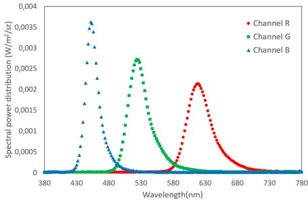
Figure 1. Spectral Power Distribution of HMD
