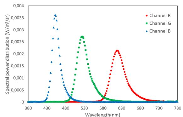
Figure 1. Spectral Power Distribution of HMD
