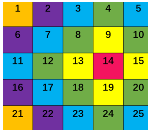
Figure 11. BFS traversal sequence (root = 14). Suppose that the most aligned sub-image is index 14, then we expand the grid to indices 9, 13, 15, 19, then to 4, 8, 10, 12, 18, 20, 24 ...
