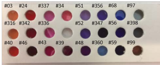
Figure 3: Color filters phantom: 23 Roscolux filters dots are glued on a cardboard slab. The empty slot is for 100% transmittance measurements.
