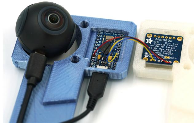
Figure 6. KVIRP's Insta360 Air, controller, and thermal imager
