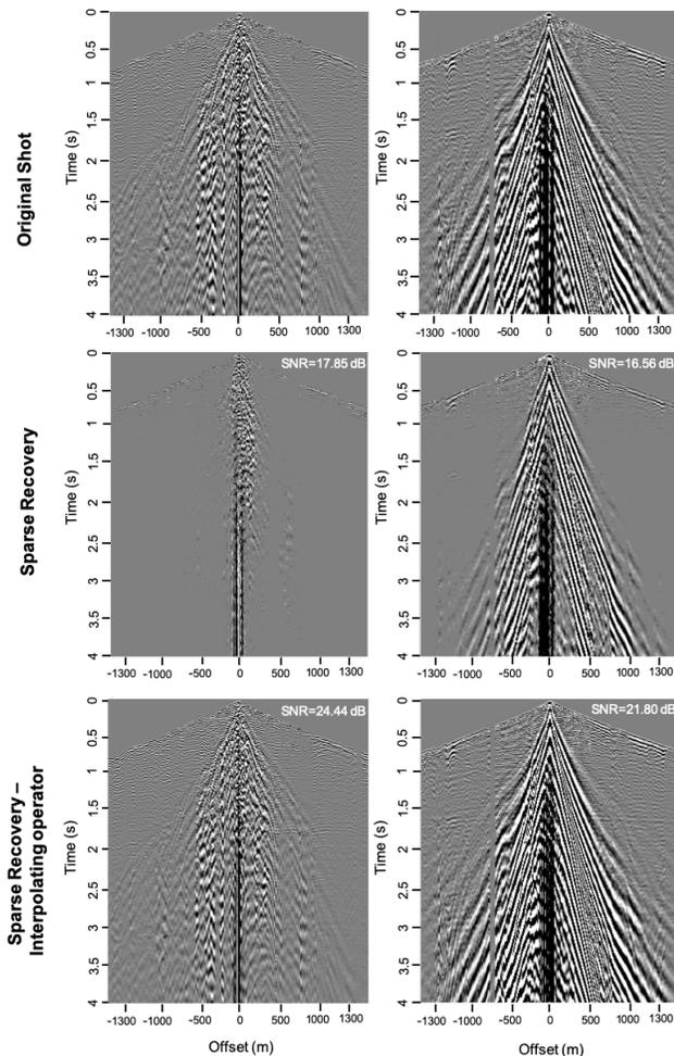
**Figure 4.** Reconstruction of 2 missing shots in a 20% compression scenario for the two sparse recovery methods.
