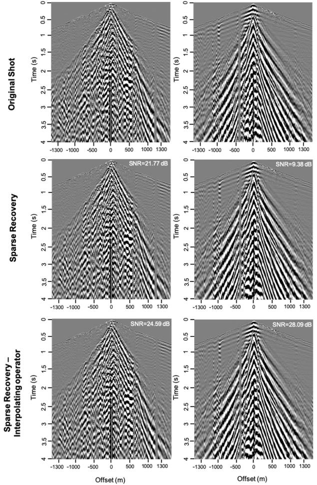
**Figure 3.** Reconstruction of 2 missing shots of a 2D wavefield in a 10% compression scenario for the two recovery methods.
