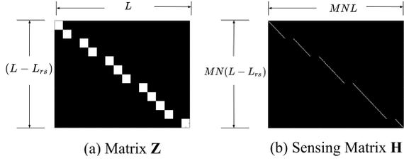
**Figure 1.** (a) Matrix  $\mathbf{Z}$  for  $L = 16$ , and  $L_{rs} = 4$  (b) sensing matrix  $\mathbf{H}$  for  $M = 4$ ,  $N = 4$ ,  $L = 16$ , and  $L_{rs} = 4$ .
