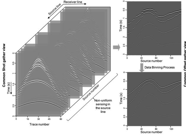
**Figure 2.** Synthetic seismic data. The common shot gather view shows the nonuniformly sampled data in the source line. The irregular data recasting onto a regular grid destroys the continuity along the arriving wavefronts in the top common offset gather. In the bottom common shot gather, the binning process cast the irregular sampled data into a regular grid to maintain the continuity.
