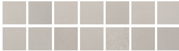
Figure 2. Images of paint and fabric samples removed from their scene context. The top row is matte white paints: Ace Premium, Ace Rust-Oleum, Krylon ColorMax, Liquitex, Rust-Oleum, Rust-Oleum 2X, and Colorshot. The bottom row is fabrics: Wool, Felt, Cotton, 97% Cotton 3% Spandex, Silk, 60% Cotton 40% Polyester, and Polyester.
