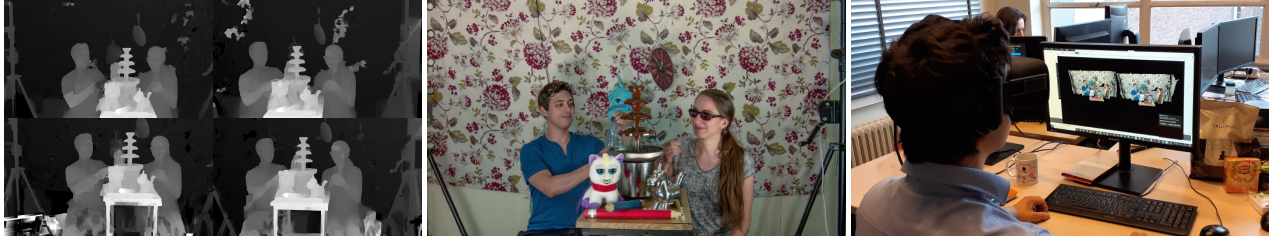
Figure 3. (a) 4 \times 4 depth maps, (b) synthesized virtual view with DIBR/RaViS, (c) real-time, image-based 6DoF VR
