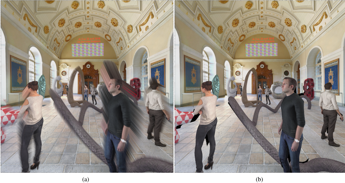
Figure 6. Museum dataset, 4 blended input views. (a) Without discarding the elongated triangles. (b) Discarding the triangles results in few disocclusions depending on the input cameras' pose. Deep black regions are disocclusions that are not covered by any input camera view and are left unpainted.
