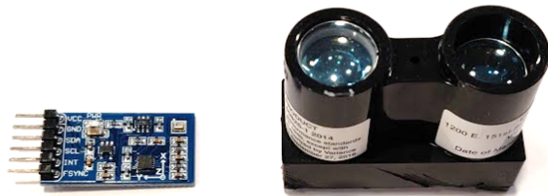
Figure 1. WaveShare 10-DOF IMU sensor (left) and time-of-flight 1D Lidar distance sensor (right)
