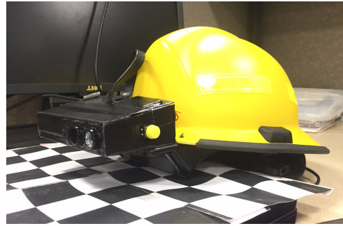
Figure 2. The Hyper-Reality Helmet prototype that the sensors are embedded into standard firefighter’s helmet
