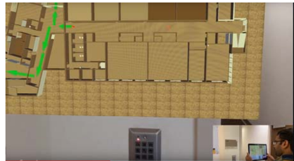
Figure 7. Spatially contextualized emergency exit locations via tablet
