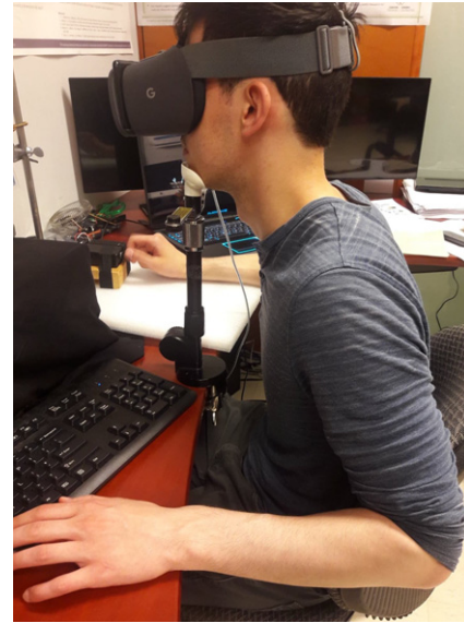
Figure 3. A picture of the setup for Experiment 1. Observers estimated slant by adjusting a line with a knob in their right hand. They registered their response by keyboard press on their left hand. A chinrest stabilized their head.
