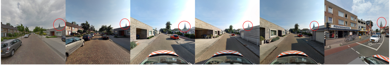
Figure 3: Example of retrieval failure due to salient features. The first image (from left to right) depicts the query location. The remaining five images show the highest-scoring matches. Out of these, only the first match is correct. The remaining matches depict locations further than 25 meters. All matches contain the same church steeple (circled in red) as a salient feature.
