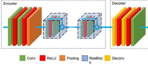
Figure 1: The architecture of the proposed over-exposure correction network (OEC).
