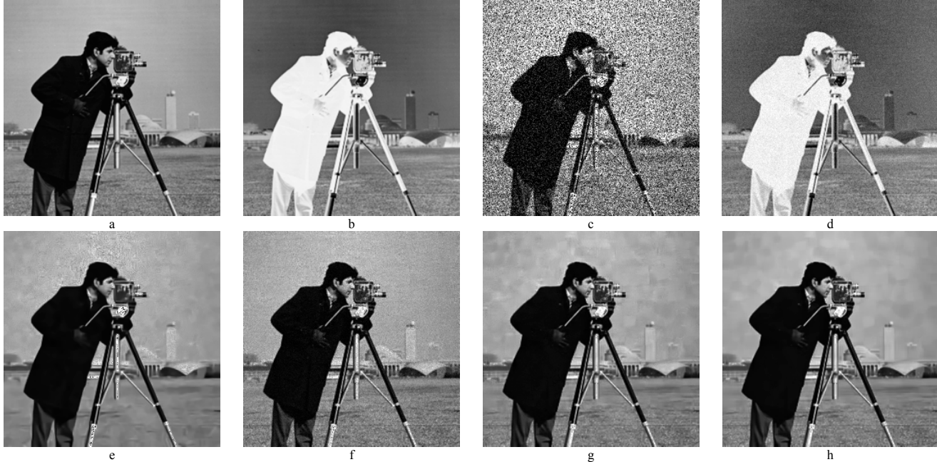
Figure 3. Channel #25 of test image: a) true phase, b) true amplitude, c) noisy phase, \sigma=0.5 , SNR_{\phi} = 0.7 dB, d) noisy amplitude, e) BM4D, SNR_{\phi} = 13.3 dB, f) CCF, SNR_{\phi} = 16.2 dB, g) ImRe-BM3D WI, SNR_{\phi} = 19.6 dB, h) ImRe-BM3D IT, SNR_{\phi} = 20.9 dB
