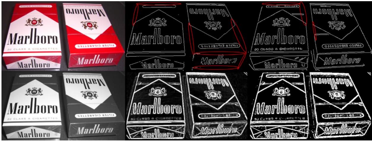
Figure 7. (a) Original image, (b) Sobel filtering, (c) Canny edge, (d) Gray image, (e) Proposed method (gray scale), (f) Proposed method (binary)
