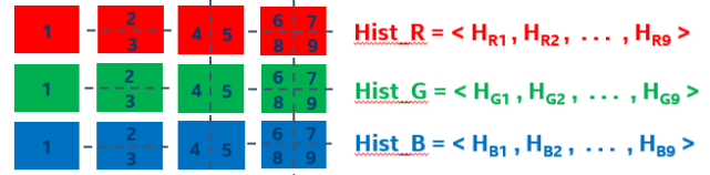
Figure 3. Illustration of algorithm based on spatial pyramid of color histograms. Best viewed in color.
