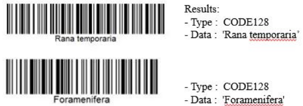
Figure 10: Decoding results from the Pyzbar package with the different types of barcodes.
