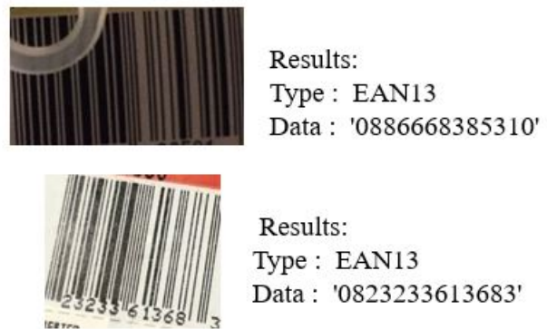
Figure 11: Decoding results from the Pyzbar package with the detected barcode region.
