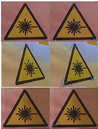
Figure 4: Typical result of the SURF detector ( OpenSurf ) - only a very little number of keypoints can be detected.
