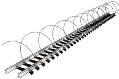
Figure 5: Helix-like trajectory of the laser scanning spot while driving.
