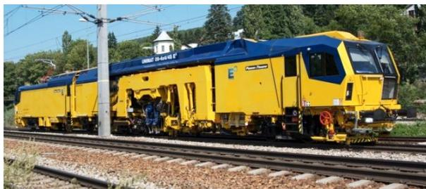
Figure 1: A typical tamping machine during work.
