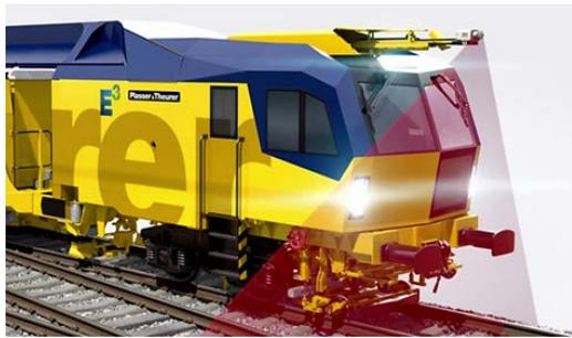
Figure 3: Tamping machine with a roof-mounted 3D laser scanner.
