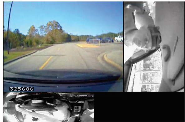
Figure 1. Example of composite video frame. In this case the rear camera is not used, resulting in a blank image for the lower right pane.
