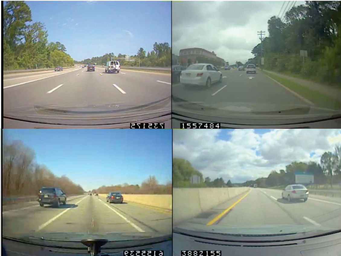
Figure 5. Comparison of two vehicles from early and late in the study. The top left shows a frame from early in the study for a vehicle with stable extrinsic parameters; the top right shows the same vehicle but late in the study. The left image is mirrored to show how well it orients with the same features in the bottom of the right image. In contrast, the bottom two frames show a different vehicle early and late in the study, where the camera has clearly shifted orientation, as shown by the misalignment on the features at the bottom of the frames.
