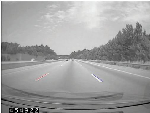
Figure 4. Lane markings located by directed Hough transform.
