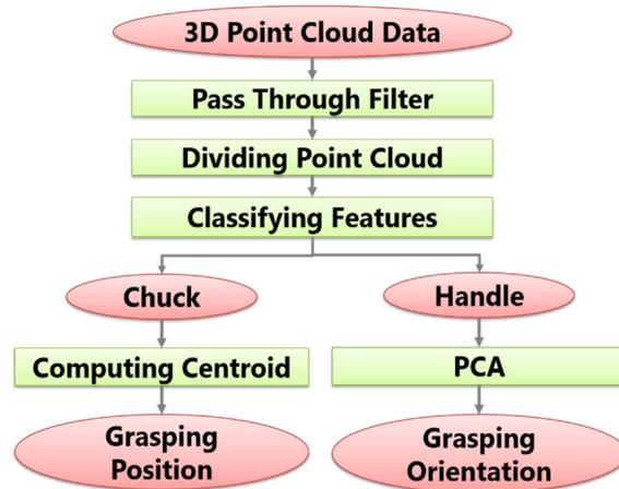
Fig. 2. The flow of processing 3D point cloud data
