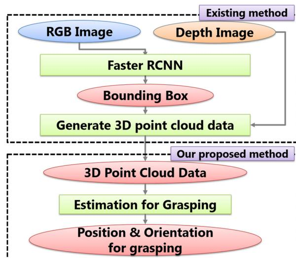
Fig. 1. The entire flow of estimating the position and orientation of the drill.
