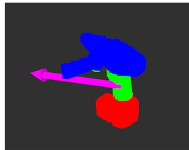
Fig. 7 The estimation error of the orientation of type-B drill. The pink colored arrow indicates the estimated orientation of a drill. The blue part is the chuck of the drill.
