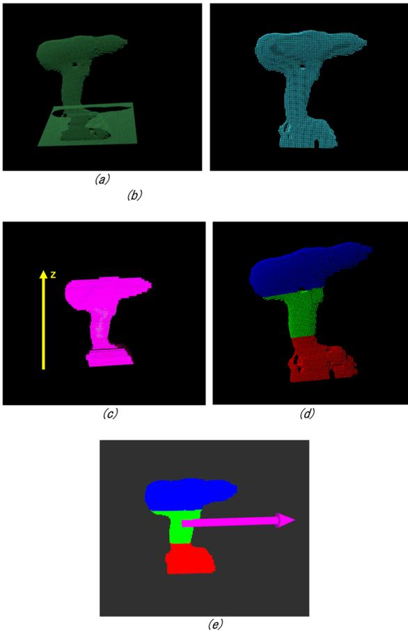
Fig. 3 The processing of the 3D point cloud data
