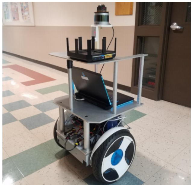
Figure 1. The experimental robot platform used to evaluate the proposed localization techniques. At the top is a Kodak PixPro sp360 4K omnidirectional camera placed on top of a Velodyne VLP-16 3D LiDAR. A TPLink Talon AD7200 60 GHz millimeter wave router is located on the top shelf. A Decawave DW1000 UWB transceiver is mounted on the top shelf visible underneath the VLP-16. An Alienware 15 r4 laptop handles localization inference and navigation.
