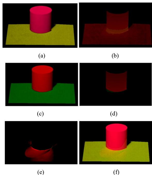
Figure 5. Component images (a)-(e) produced in the reconstruction process and the construction result (f). (a) Diffuse reflection, (b) interreflection, (c) luminescence by direct illumination, (d) luminescence by indirect illumination, and (e) interreflection by fluorescent illumination.
