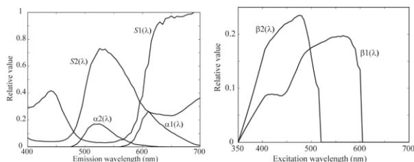
Figure 4. Spectral curves of reflectance and emission functions (left), and excitation functions (right) for the two fluorescent objects.
