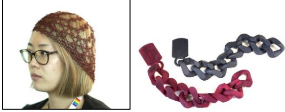
Figure 7: On the left, a dyed head piece. On the right, a reference part used to evaluate the viability of different colored dyes.
