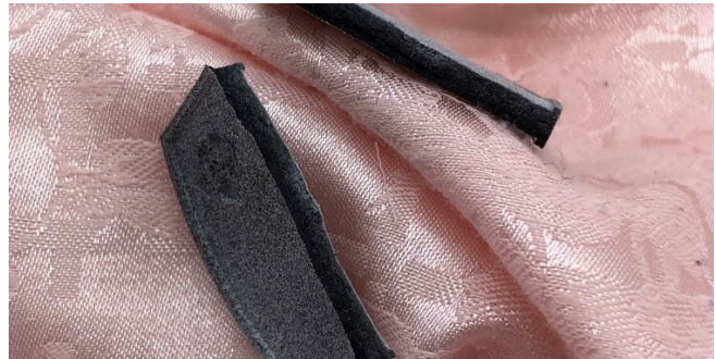
Figure 1: A Multi Jet Fusion part broken in half, showing the grey appearance of the surface as well as the dark black color of the interior.
