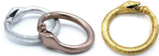
Figure 5: On the left are the spray coated bracelets, and on the right is the gold-leaved sample.
