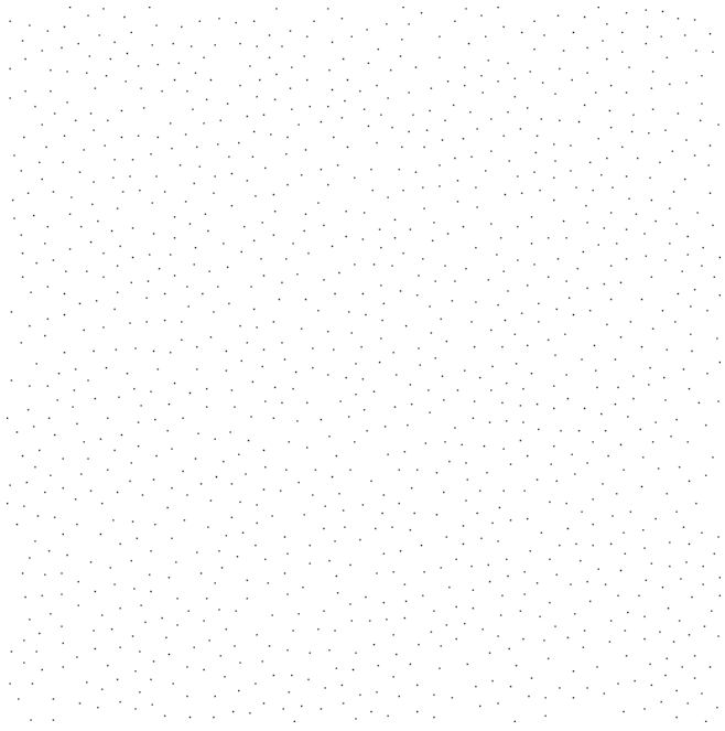
Figure 2 Signal carrying artwork obtained by marking the locations of the local minima of the watermark signal, with keep out criteria around each point to achieve a more uniform distribution.
