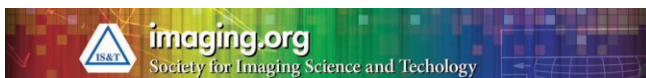
Figure 1 Example of an image with multiple artistic patterns in the background. Here either the pattern of vertical lines or the colored squares may be used to covertly carry a signal without changing the appearance of the image.
