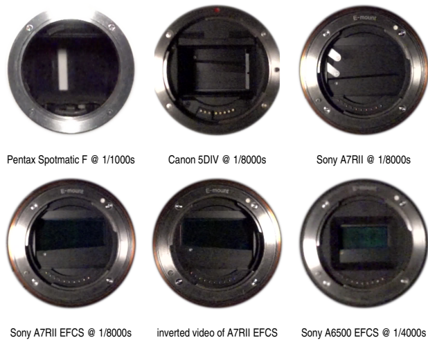
Figure 5. High speed images of focal plane shutters
