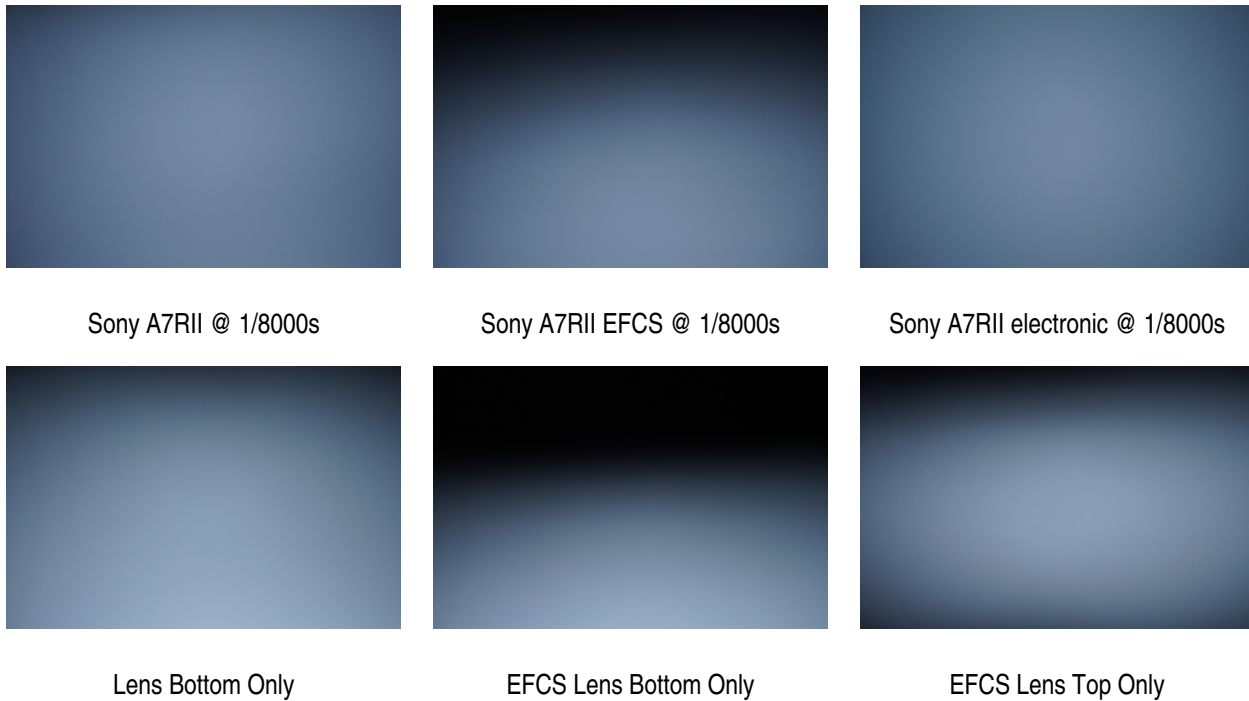
Figure 7. Shading by focal plane, EFCS, and electronic shuttering
