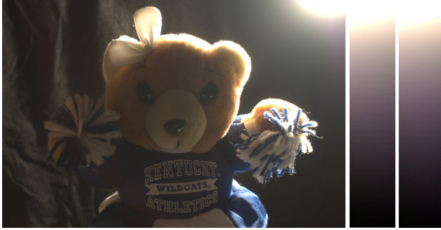
Figure 5. RX100 V image with stripe artifacts, enlargement, and repair
