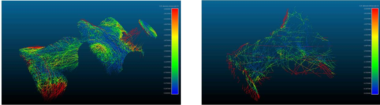
**Figure 9.** Scans colored with point to point distance [mm] to reference scan. The coloring scale varies from 0 to 3 mm. Left: Calibration with 6 spheres and scan with 300 crosses (relative to Fig. 6 top, scan 6), Right: Calibration with 3 spheres and scan with 150 crosses (relative to Fig. 6 bottom, scan 3).
