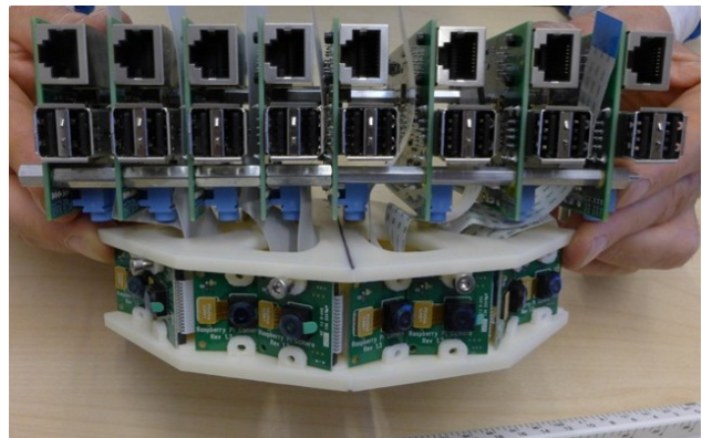
Figure 7: Camlot camera prototype with RPI boards
