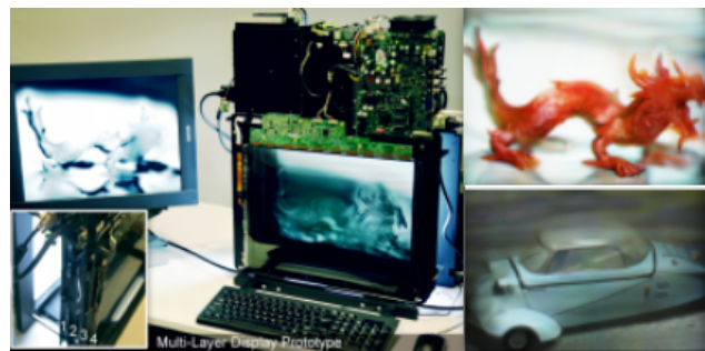
Figure 14. Lanman - Polarization fields: dynamic light field display using multi-layer LCDs [118].
