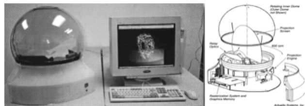
Figure 11. Favalora - Volumetric three-dimensional display system with rasterization hardware [107].
