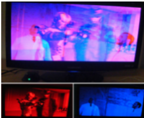
Figure 7. Inexpensive 3D Stereo for Two Users Using a Single Display [57].
