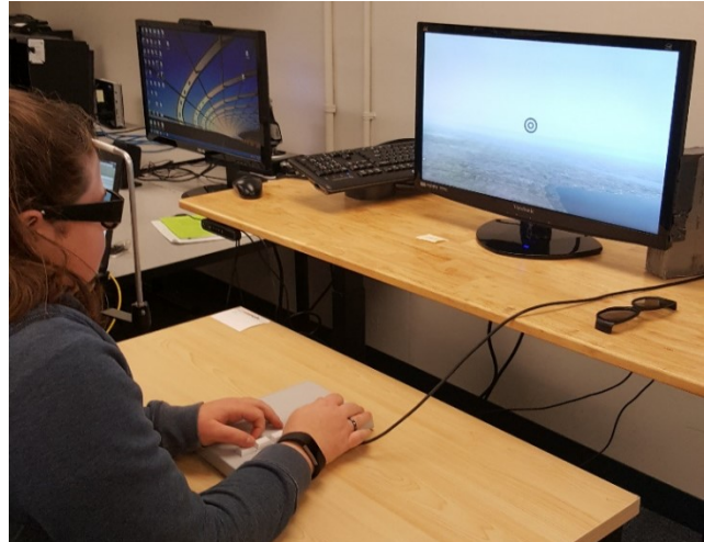
Figure 4. Depth discrimination experiment apparatus. Participant eye height remained fixed using a head/chin rest attached to the small table in the foreground. The height of the monitor relative to the eyes was controlled using the adjustable height table supporting the display.
