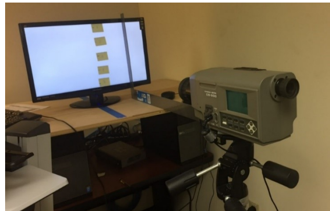
Figure 5. Apparatus used for measuring crosstalk on the ViewSonic display. Measurements were made with either the left or right lens of the polarized 3D glasses positioned in front of the chromameter lens.
