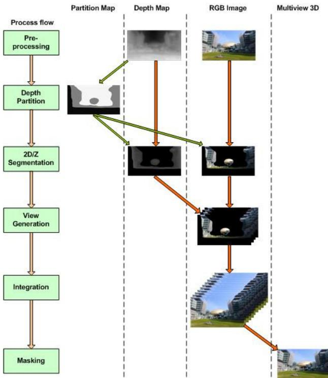
Figure 2. Dynamic multi-view autostereoscopic display with 2D+Z format input
