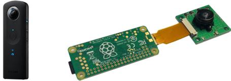
**Figure 1.** Environmental light acquisition hardware. Left: 360° Ricoh Theta camera used for the server solution. Right: Raspberry Pi Zero and 180° fisheye camera used in the edge solution.
