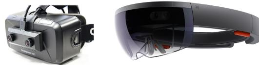
**Figure 4.** AR Units. Left: Oculus Rift DK2 with mounted OvrVision Unit. Right: Microsoft Hololens.
