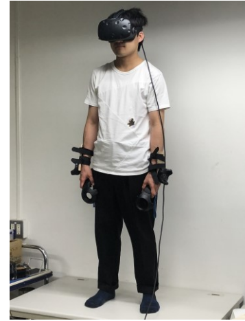
Figure 2. Experimental device: HTC Vive head mount display, tracker and controller were used in the experiment
