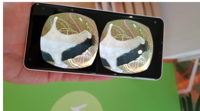
Figure 16. Burning-in effect observed on the OLED displays of the Google Pixel 2 after three months of use.
