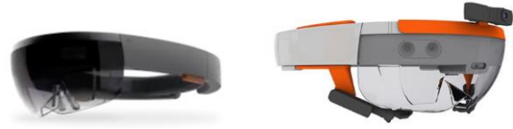
Figure 2. AR headset and an eye tracking add-on for AR headsets.
