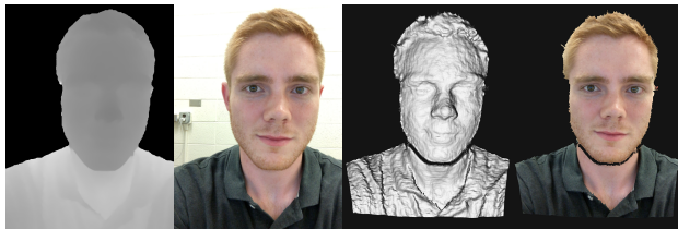
Figure 2. Example frame as captured by the Acquisition Module on an iPhone X. From left to right: a depth map, Z ; the depth map's corresponding color texture image, C ; the 3D geometry frame reconstructed from Z ; the 3D geometry frame mapped with its color texture image.
