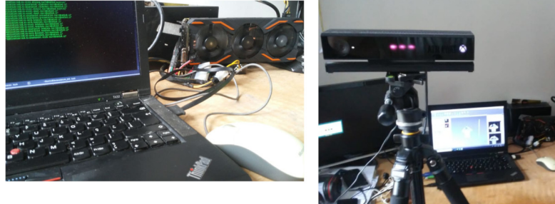
Figure 5: Left: Partial view of the notebook with an external GPU attached; Right: Kinect 2 connected to the notebook computer used for capture outside the laboratory (right).
