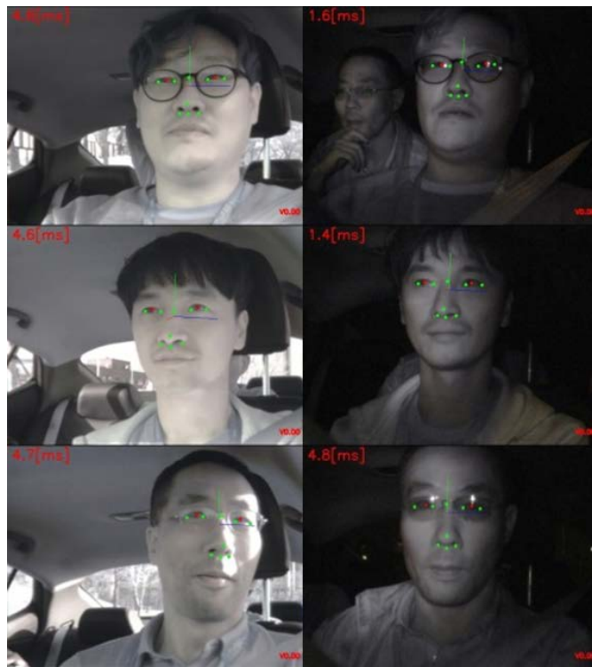
Figure 4. Driver pupil tracking on RGB (left) and NIR (right). Red dots indicates the tracked center of the pupils
