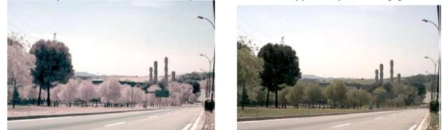
Figure 2. Image captured without IR-cut filter (L) and with IR-cut filter (R) [1]
