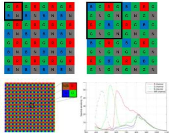
Figure 1. RGB-IR sensor patterns and their typical spectrum [6]
