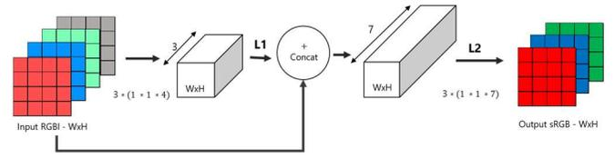
Figure 7. CNN model color correction flow
