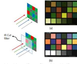
Figure 6. (a) without IR-cut filter (b) with IR-cut filter
