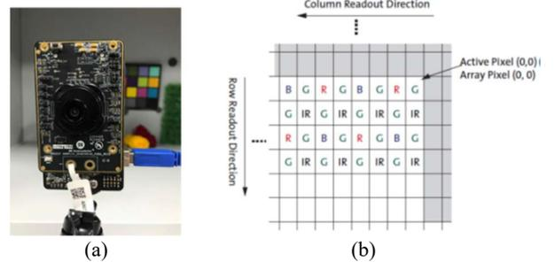
Figure 8. (a) AR0237CS Camera kit (b) 4x4 RGB-IR Bayer pattern
