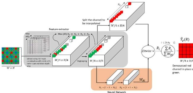
Figure 5. CNN model for demosaicing
