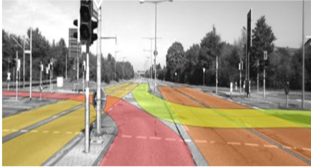
Figure 4. Example of a complex lane crossing scenario. Figure is reproduced from KITTI. The red demonstrates the DriveSpace of a car turning left, the orange shows the drivespace of a vehicle driving forward. Yellow would be the DriveSpace of other vehicle.
